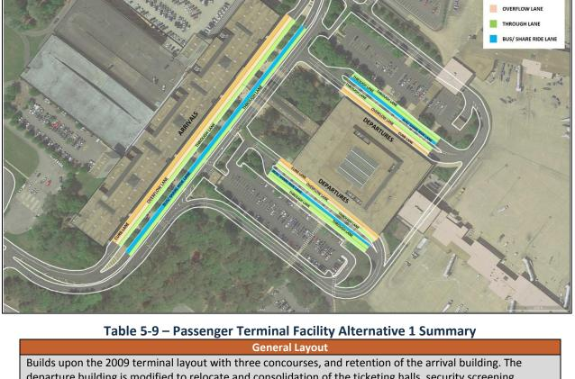
Figure 5-10 – Existing Terminal Curbside Layout
