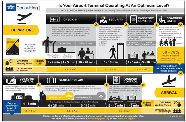
Figure 4-5 – Passenger Terminal Through Process
